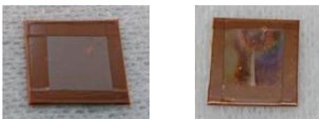
Fig. 1 Pictures of Cu samples deposited with a 10 nm TiO<sub>2</sub> film before Rh plating (Left) and after plating (Right).
