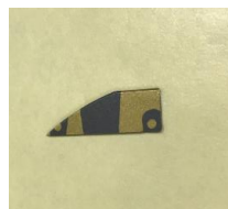
Fig.2 Image of InP small piece deposited with AuGe/Ni/Au.
