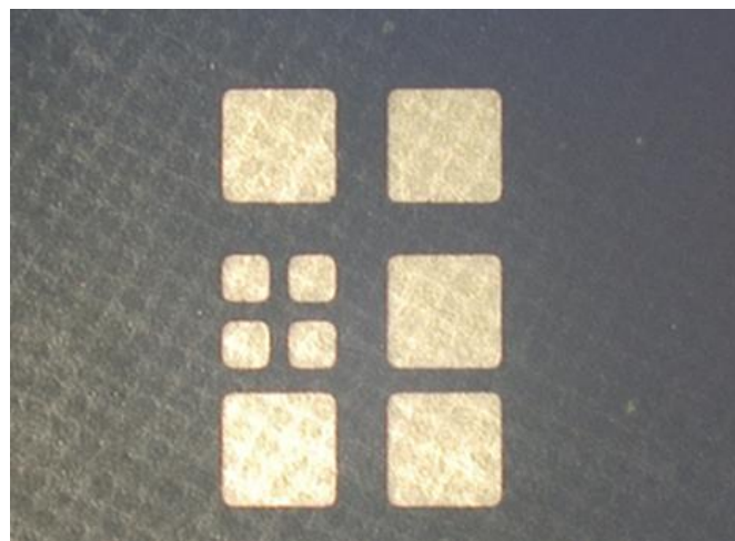
Fig. 1 Photograph of alignment marks on printed circuit board.
