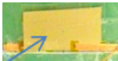
Fig. 2 Photograph of the PVDF film with conductive nanoink
