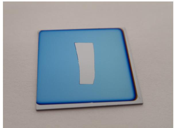
Fig. 1 Deposited BaTiO<sub>3</sub> thin film.
