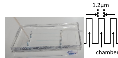
Fig. 2 Microfluidic device and chamber dimensions.
