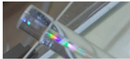
Fig. 1 Varied-line-spacing grating on the glass mandrel.
