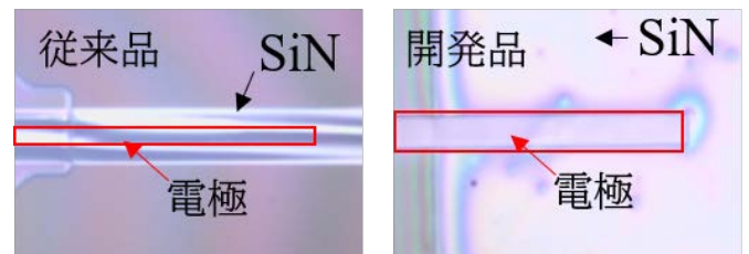
Fig.1 CCD images of comparison between developed MEMS chip (right) and conventional one (left).
