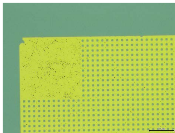
Fig. 2 Image of the gate electrode pattern after lift-off of Au
