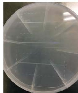
Fig. 1 Pictures of ultra-short-period transmission gratings fabricated by metal mask process.
