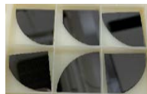
Fig. 1 Appearance of 1/4 Si chips after dicing.
