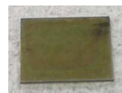
Fig. 2 Appearance of SiC chip after dicing and followed by the growth of GaN.
