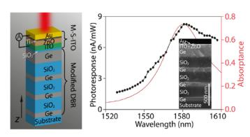
The first experimental results of TP coupled hot-electron photodetector.
