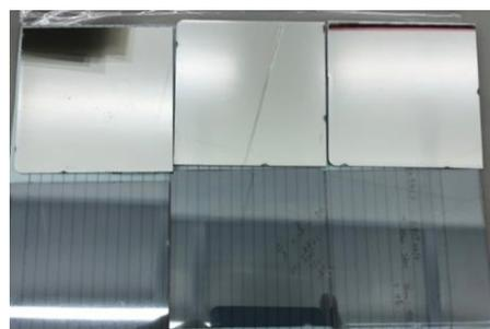
Fig. 1 Ag- deposited PC sample: 100 nm thick (top) and 15 nm thick (bottom).
