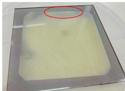
Fig. 2 15 nm thick Ag-deposited PC sample after Ag etching.
