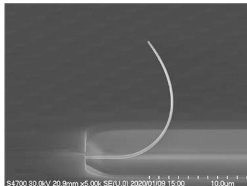
Fig. 1 SEM image of vertically curved Si waveguide
