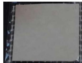
Fig. 2. W-CVD film appearance after adhesion tape test
