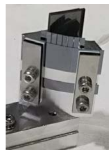
Fig. 1 Fabricated X-ray multi-beam optics with hyperboloidal holder.
