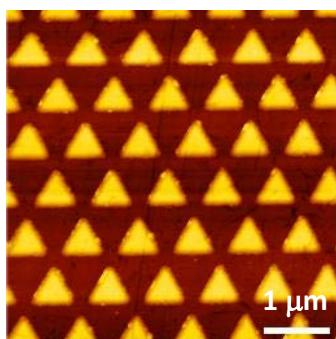
Fig.1 AFM image of periodic arrangement of permalloy ( $Ni_{78}Fe_{22}$ ) nanomagnets with three-fold rotational symmetry.
