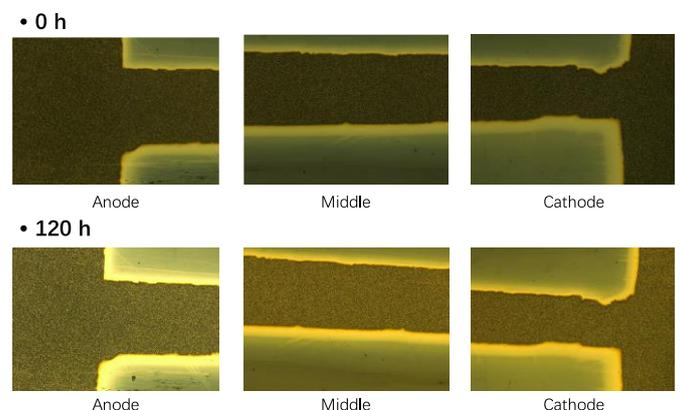
Fig. 1. The morphology change of the sample after EM test
