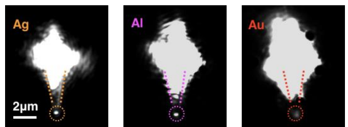
Figure 2. optical image of fabricated aluminum triangular structures with white light illumination to slit structures. Materials are aluminum, silver and gold from left to right.
