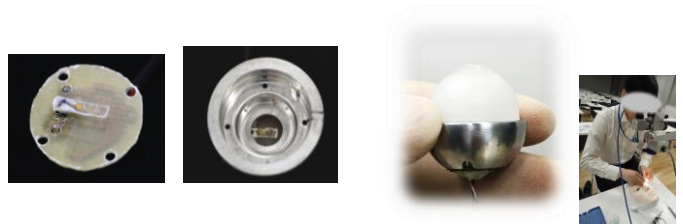
Fig. 1 Cap of retinal force sensor. Fig. 2 Eye ball model.
