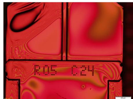
Fig. 2 Optical microscope image of cantilever covered with photoresist.
