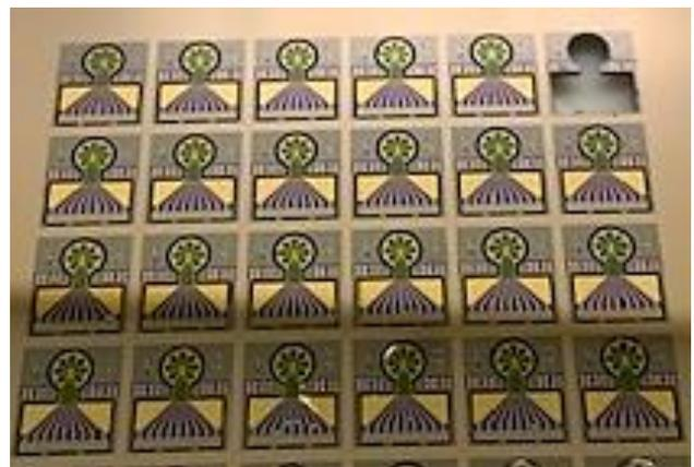
Fig. 1 An image of microcalorimeter devices composed of TES arrays and optical cavities on a Si substrate cut by deep RIE.
