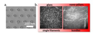
Fig. 1 a) SEM image of nano-pillar after patterning and lift-off process. b) The effect of kinesin patterning on MTs coordinate behavior.
