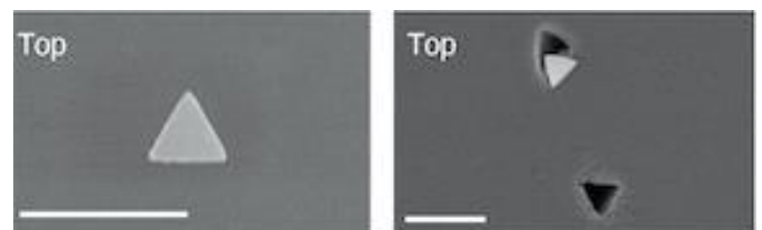
Figure 2. (Left) Triangular Pt nanocatalyst prepared by using E-beam lithography and E-beam evaporation of platinum. (Right) Top view after the etching with the triangular Pt nanocatalyst. Scale bars indicate 1 \mu m.
