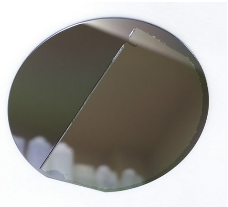
Fig. 1 Photo of wafer-bonded III-V-OI wafer after etching InP substrate.
