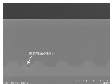
Fig. 2 SEM images of sample without phosphoric wet etching
