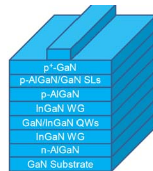
Fig. 1. Schematic structure of GaN laser diode fabricated for present study.
