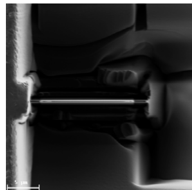
Fig. 1 SIM image of Si sample thinned by FIB fabrication
