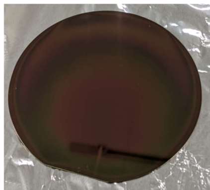
Fig. 1. Picture of Si wafer with 5 \mu\text{m} of SiN film.
