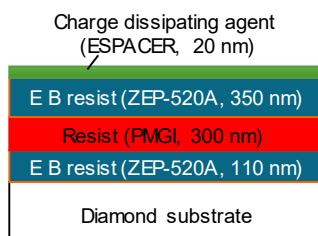
Fig1. Schematic cross sectional structure of triple resist layer for T shaped gate fabrication process.
