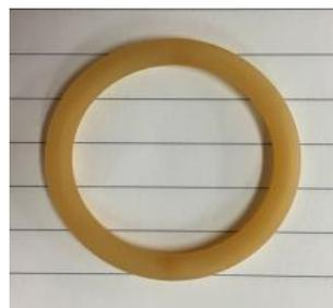
Fig. 1 Picture of a fluoroelastomer O-ring.
