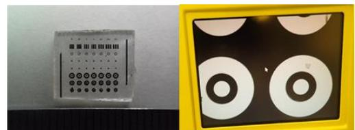
Fig. 2 Devices after depositions of Al<sub>2</sub>O<sub>3</sub> / electrodes.
