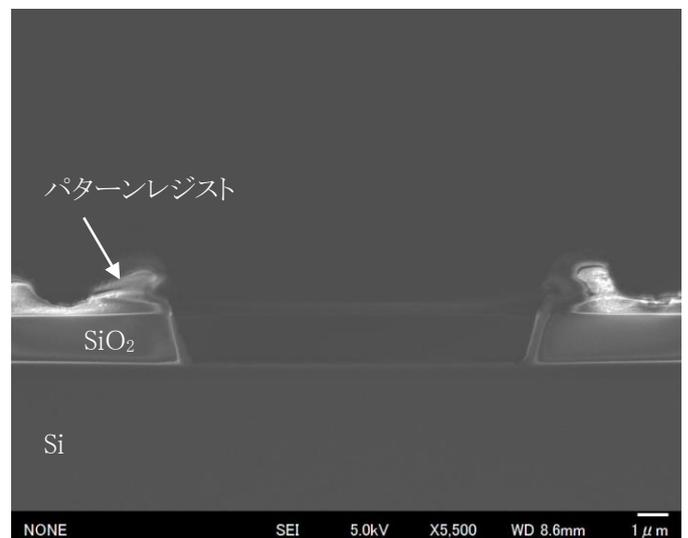
Fig. 1 SEM cross-sectional image of SiO<sub>2</sub>.
