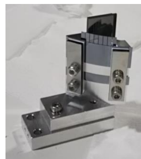
Fig. 1 Fabricated short-focal-length X-ray multi-beam optics with hyperboloidal holder.
