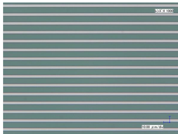
Fig. 1 A developed resist pattern with L/S = 5 \mu\text{m} / 10 \mu\text{m} .
