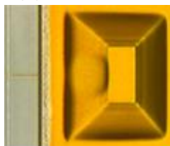
Fig. 1 (a) Top view and (b) enlarged view and (c) height profile of polymer micro mirror in the cavity.
