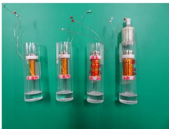
Fig. 1 A prototype of impact vibration power generator studied in this work.
