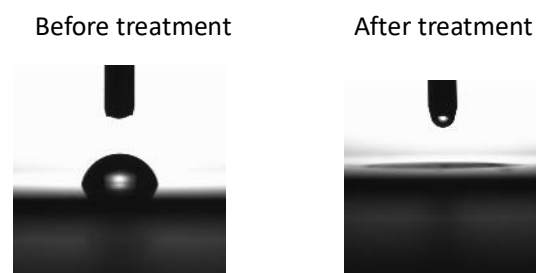
Fig. 2 Water contact angle measurement before and after \text{O}_2 plasma treatment
