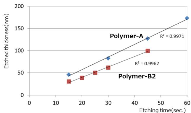
Figure 1. Experimental results of dry etching durability by using each polymer samples
