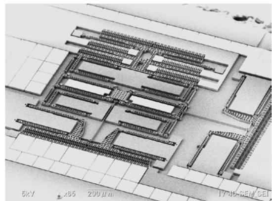
Fig.1 SEM image of 3D microstage
