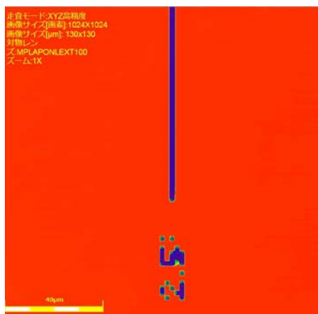
Fig. 1. Laser microscopy image for trench structure.
