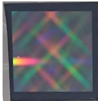
Fig. 1 A prototype of 20 mm X 20 mm device fabricated by electron beam lithography F7000S
