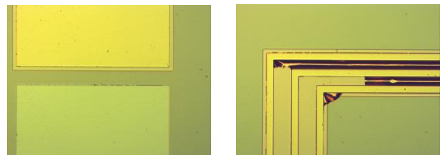
Fig. 2 Photograph of electrode after lift-off.
