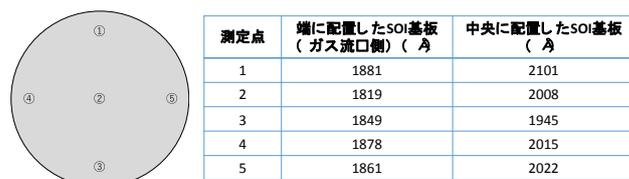
Fig. 1 Sampling points for SiN film thickness measurement.
