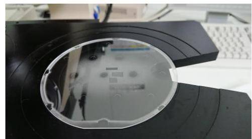
Fig. 1 Sapphire wafer after Etching.
