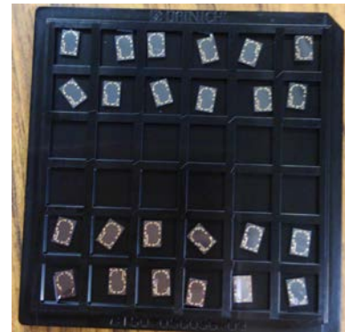
Fig. 2 Integrated LSI-MEMS tactile sensor
