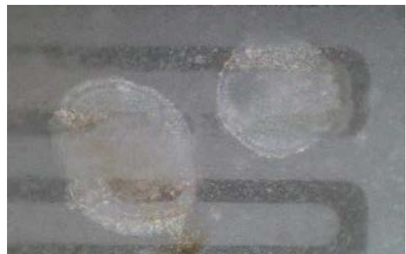
Fig. 2 Pictures of SiO x 1.5 μm sample after high temperature / high humidity current test 550 h
