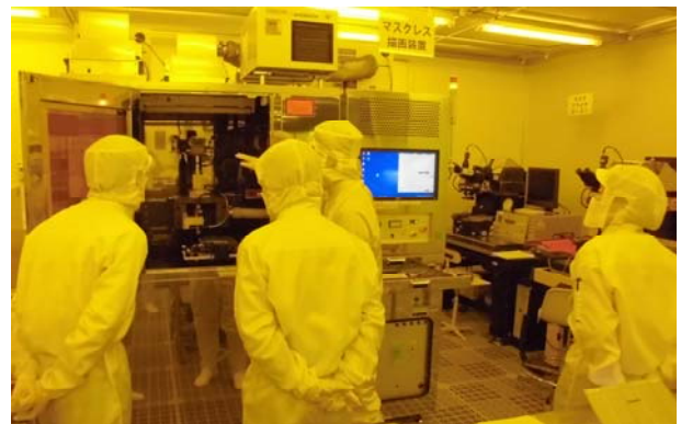
Fig. 1 Explanation of maskless exposure equipment.
