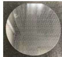
Fig.1 Silicon wafer after etching
