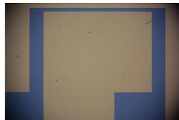
Figure 1. Au film patterning by a liftoff process.
